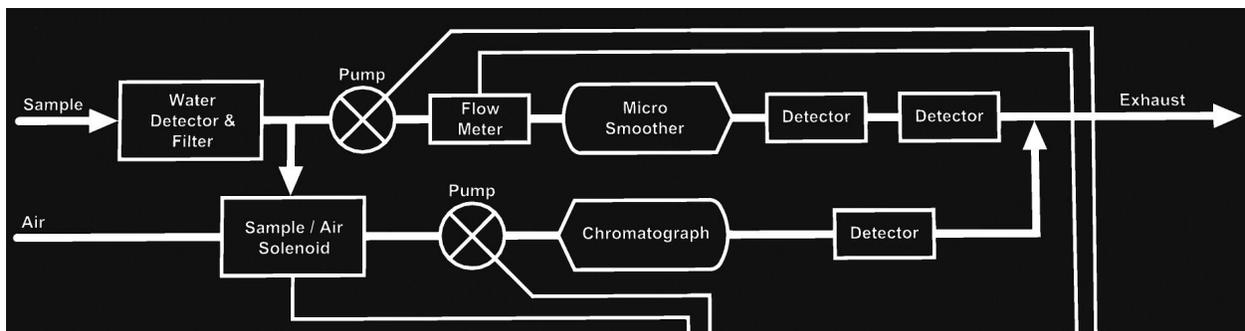
2) SAMPLING MECHANISM: Taking into consideration the "snapshot" concept described above, this is accomplished by having a solenoid in the Bloodhound
